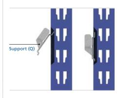
After inserting the four supports, attach the shelf by applying light pressure to each corner until it is secure.
