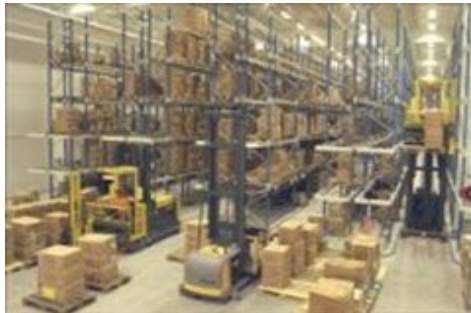
A typical VNA Installation
